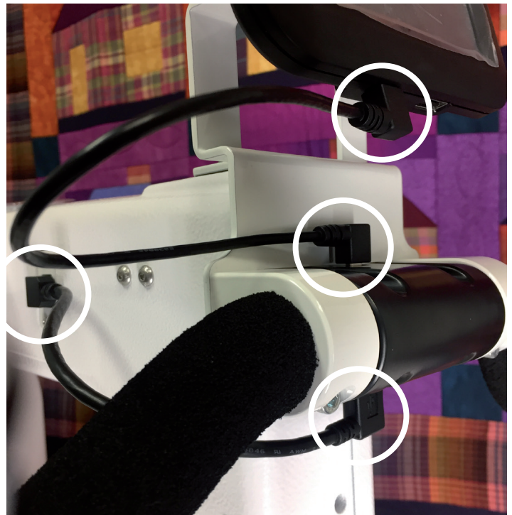
Top cable: handlebar to display QM23010; Bottom cable: handlebar to machine QM23011.
