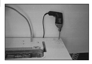
7. Put the light cord and the goose neck light into the pre-drilled hole. Put a male plug end on the cord and plug into the back of the motor. This is a six volt outlet so be sure and use the bulb supplied with the machine.
