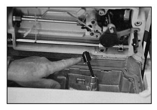
10. Slide the hinges into the back of the machine onto the oil pan assembly and add oil to the fill lines marked on the pan.
