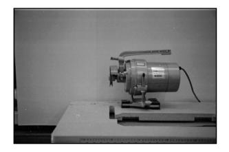
2. Mark around the motor mounts, and drill 5/16" holes through the table be careful not to break out the laminate on the top of the table when drilling through.
