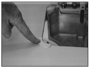
8. Now, turn the table upright. Slide the oil pan rubber corners onto the oil pan and set the pan into the table.
