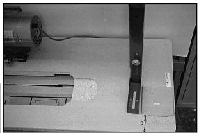
6. Drill an 11/16" hole in the right rear of the table, being careful not to drill into the wires from the switch to the motor on the underside of the top. This hole is for the thread stand.
