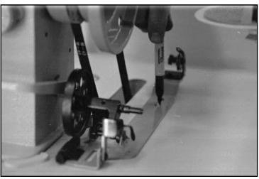
Do not over fill the bobbin. The optimum length of thread will fill about 80% of bobbin capacity. This can be adjusted by Adjusting Screw (E) of Bobbin winder stop latch.
