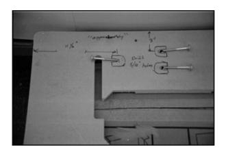
3. Treadle, clutch arm and a treadle bracket is shown here. Use a bracket on each side of the treadle to fasten it to the flat horizontal bar on the bottom of the legs.
