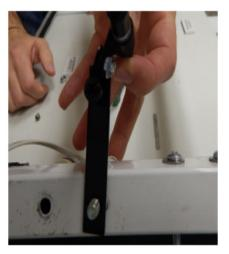
2 Secure the encoder and EZ-laser by tightening the bolt. As pictured.
