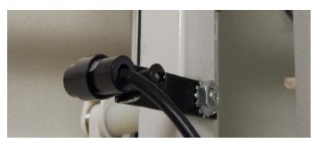
**5** Plug the laser into the laser port on the PCB box.
