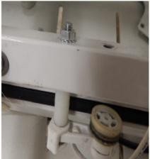
**2** Use the bolt that the encoder is attached to in order to install the EZ-laser.
