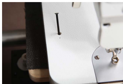
Figure 38 Oil dip stick lifted
