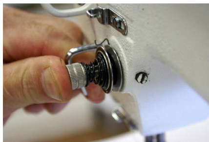
Figure 86 Press in and notice the tension disk opens
