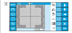
Make a duplicate of the pattern and flip it vertically. Move the flipped pattern to the top left corner of the editing screen. Make a duplicate and flip it horizontally. Move the pattern to the right top corner of the editing
