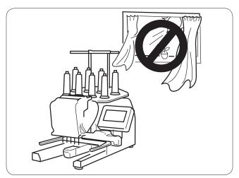
Do not expose the machine to direct sunlight or open air.
