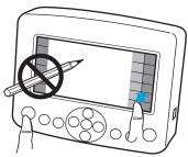
Press the LCD touch panel and buttons gently. Rough or forceful pressing may damage the unit.
