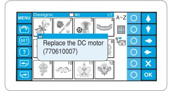
When the total running time of the DC motor reaches 1,000 hours, a message will appear advising you to replace the DC motor.
