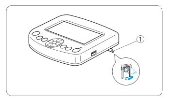
If you are using the RCS unit on the tabletop, simply insert the connector into the connector socket on the back of the machine.
