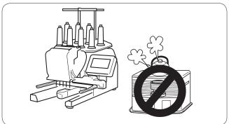
Do not use or store the machine near a heat radiator or in a place with dust or high humidity.
