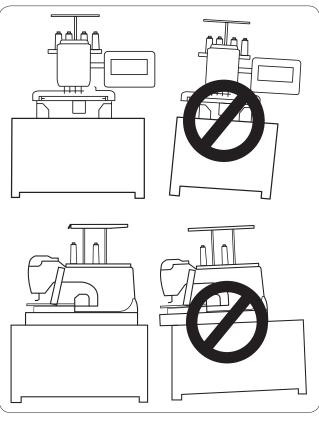
Place the machine on the flat and level surface. Make sure that all the feet firmly contact the surface.
