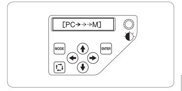
Transfer the embroidery pattern data files between the machine and PC by using optional **Digitizer MB for multi-needle**.
