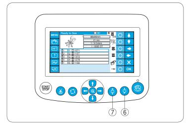
If the thread breaks or runs out while stitching, the machine will automatically stop and the hoop will go back to the position where the thread broke or ran out.
