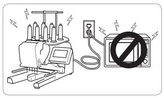
Do not use the machine near appliances that radiate electromagnetic noise such as a microwave oven, or do not plug in the machine to the same branch circuit where such appliances are connected.
