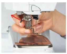
> Press the clamping lever down.
