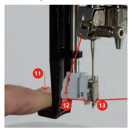
> Release the lever and the thread simultaneously to thread.
