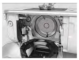
> Give one drop of oil in each of the two oil depots so that the felts are damp and make sure that the redmarked surface of the hook sleeve remains free of oil.
