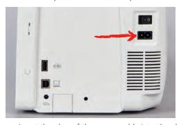
> Insert the plug of the power cable into the electrical outlet.
