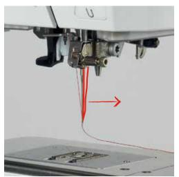
> Pull the thread under the presser foot and pull it over the thread cutter from back to front to cut.
