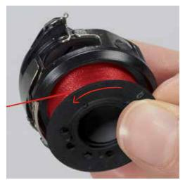
> Pull the thread into the slot from the left.
