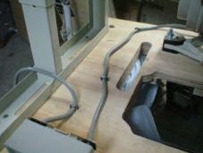
7. Install the rod onto the motor and the foot pedal, then connect the rod using the rod connector (middle part). Ensure the back of the pedal is four inches from its base, and that the clutch lever on the motor is at its highest position.
