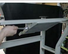
5. Mount the legs onto the underside of the table using the table screws (usually four on each side - may differ depending on machine purchased). Allow 1/2" space between the leg and the edge of the table top. Install the legs according to the marks on the underside of the table. Tighten all screws firmly.
