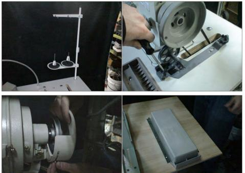
8. To install the knee-lift mechanism, insert the presser foot umbrella in the oil pan, then attach the knee-lift mechanism as shown in the photo.
