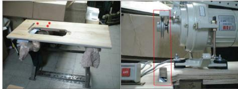
2- Install the 3 motor mount screws with a wrench, vicegrip or plyers. Your motor may differ, but installation is the same. Screws can be found in the motor box or accessories box (inside a gray pack) along with the legs.
