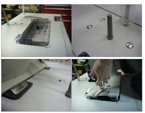
3. Locate the V-Belt and attach it to the motor pulley. You may need to tilt the machine back to place the V-Belt on the hand wheel.
